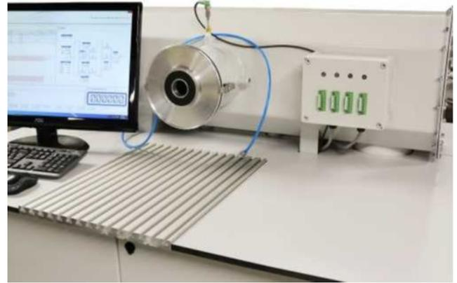
Due to the advanced nature of our test bench, a typical 3 (three) point test can be performed within 15 to 20 minutes for meters that are equipped with a high frequency pulse output.
